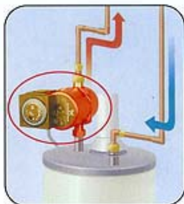
Comfort Pump installed at the hot water tank
